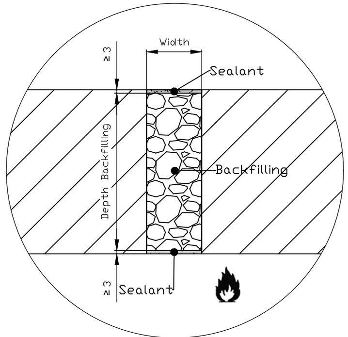
Soudafoam® FR HY backfilling at an offset of 3 mm and Firecryl® FR sealant at both sides.
