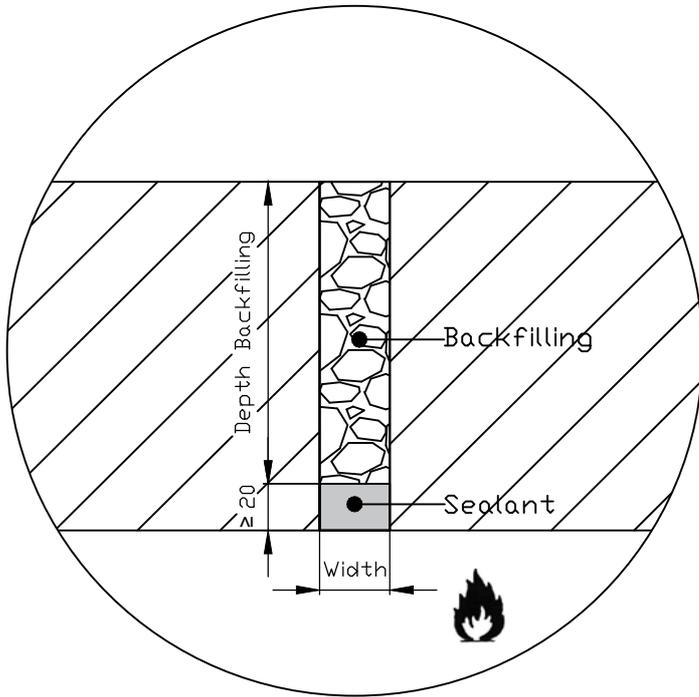
Soudafoam® FR HY backfilling flush with unexposed side and sealant at the exposed side.
