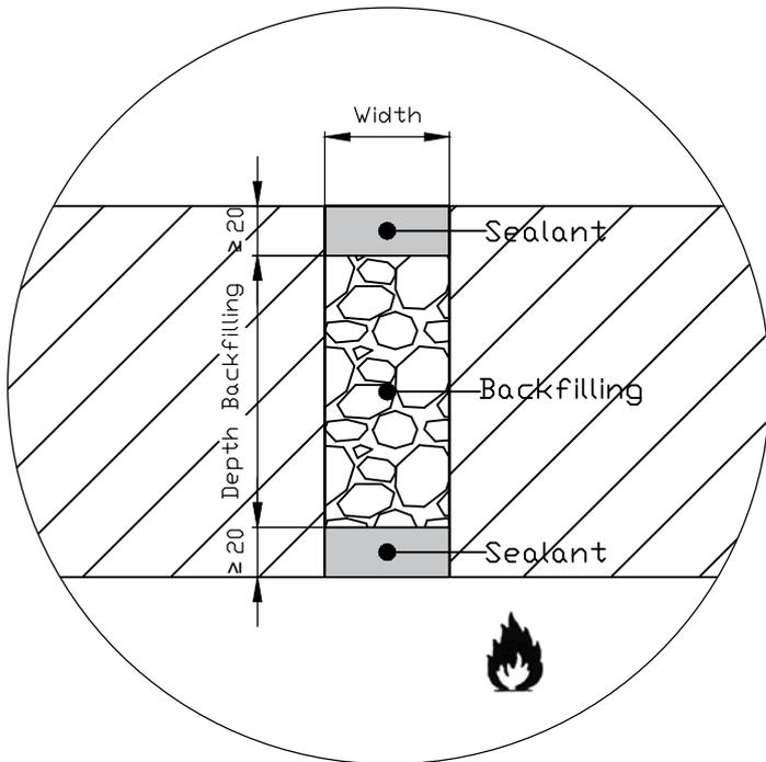
Soudafoam® FR HY backfilling at an offset of 20 mm and sealant at both sides.
