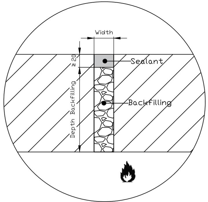
Soudafoam® FR HY backfilling flush with the exposed side and sealant at the unexposed side.
